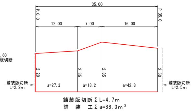
舗装版切断  $\Sigma L = 4.7 \text{ m}$
